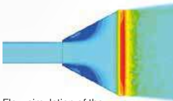
Flow simulation of the optimised blowing nozzle system
